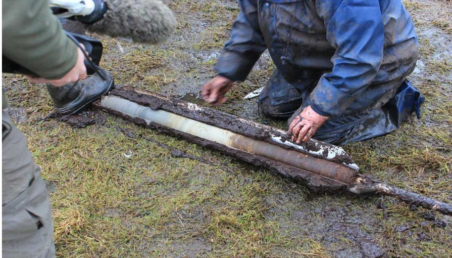
The core shown above, and below (in close-up), is from the base of the sequence. The light coloured sediment, on the left is marl from the bottom of the lake, laid down during a warm period at the end of the last Ice Age, 10,000 years ago. You can also see green layers of well preserved moss, laid down during a cold wet period. Peat cores are a powerful tool for studying the environment.
