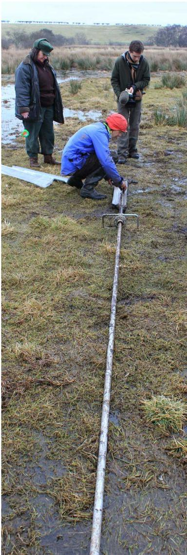
Coring is used to take column samples very many metres down into sediment layers. Each sample (each about 1m long) is taken deeper than the last, with a little overlap each time, to ensure a continuous column is produced.
